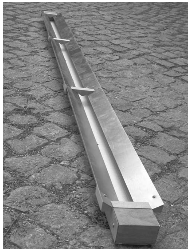
Figure 1. Photo of a seed trap installed in motorway tunnels. On top is a removable, aluminium funnel that covers a flat container of 5 \times 8 \times 190 cm. The total sampling surface area is 0.22 \text{ m}^2 .
